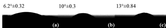
Figure 8. Contact angle measurements of (a) needle like-TiO 2 , (b) PRh, and (c) needle like-TiO 2 /PRh.
